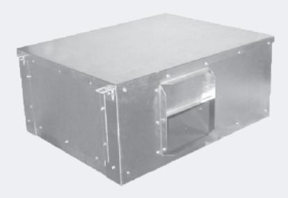
The Adirondack-Aire CC Series is a direct replacement for Singer/Climate Control CC series C revision ducted horizontal water source heat pump units. This version does not directly replace other revision code units. The CC is a complete unit that contains the compressor, blower, air side heat exchanger, water side heat exchanger, safety components, and control components.
