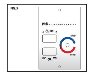
Push the control switch to the indicated 'COOL' position. For most models the room side fan will turn on. For units with factory 'cycling fan' option the room side fan will not turn on until the thermostat calls for cooling.
