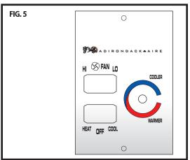
Push the control switch to the indicated 'COOL' position. For most models the room side fan will turn on. For units with factory 'cycling fan' option the room side fan will not turn on until the thermostat calls for cooling.
